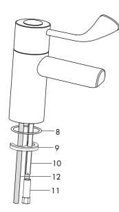
The Intatherm thermostatic basin tap is designed for installing on one hole basins.
